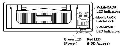
VPM-6248T Front Panel with the MobileRACK
